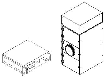
Coating box is not hermetically sealed, but is tight enough to be filled with nitrogen or another inert gas during dip cycle. Gas inlet and outlet are provided on the rear side of the device. Six M4 threads in the back cover and 16 M4 threads in the ceiling of the coating box are available to attach other equipment inside the box e.g. uv curing lamp, heat curing furnace.
